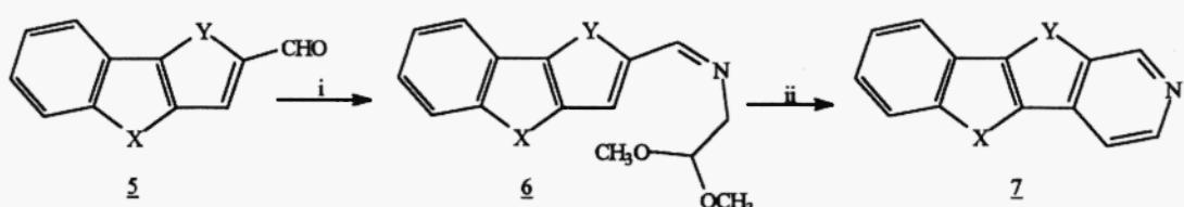
Reagents and conditions : i, NH<sub>2</sub>CH<sub>2</sub>CH(OCH<sub>3</sub>)<sub>2</sub>, toluene, azeotropic reflux ; ii, polyphosphoric acid, 150°C.
